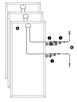
Attach the bare-wire ends of the MC4-to-Bare Wire pair • to the charge controller •. The red wire connects to the (+) input and the black wire connects to the (-) input.
