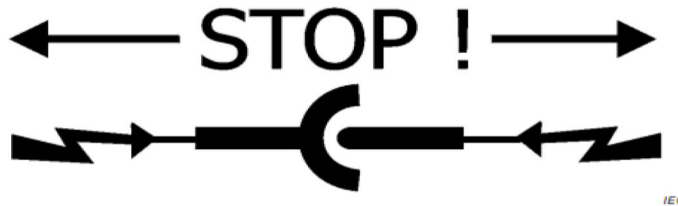
Figure A.1 – Symbol "DO NOT DISCONNECT UNDER LOAD"
